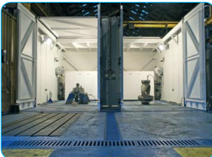
• 2 High Pressure test booths with doors open & one roof retracted
